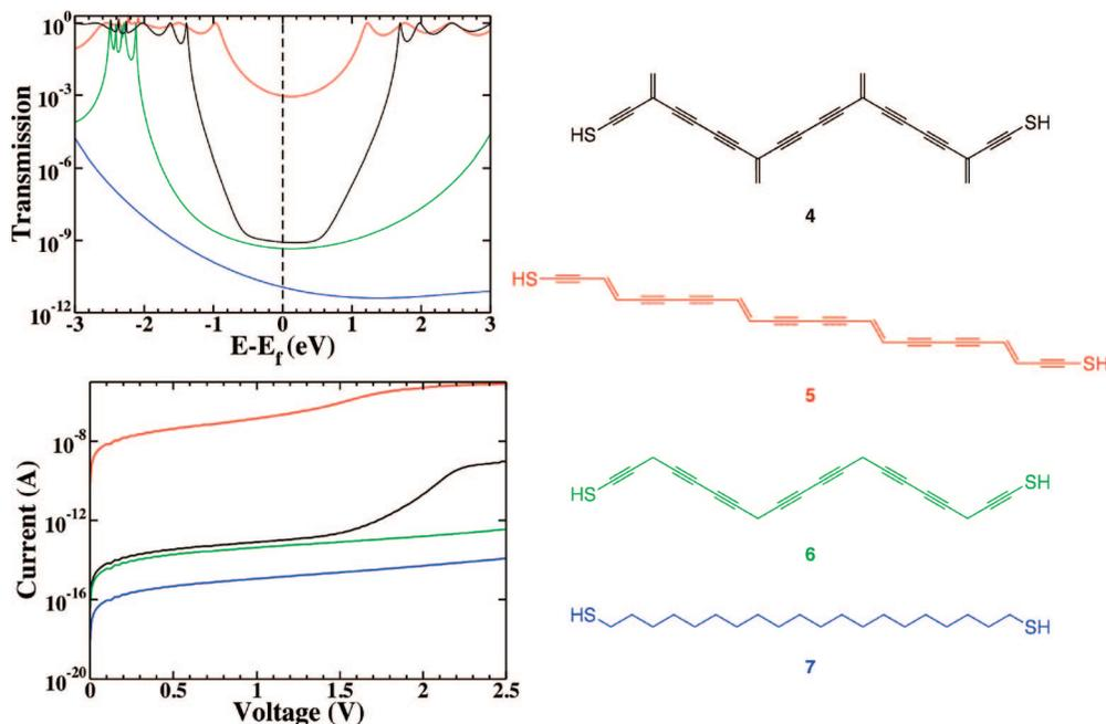
**Figure 5.** Zero bias transmission as a function of energy, and current as a function of voltage, for a group of comparable molecules, illustrating the unusual transport characteristics of a cross-conjugated system. Specifically, an extended cross-conjugated molecule (**4**) is compared with its linearly conjugated counterpart (**5**) and with a partially conjugated (**6**) and a saturated (**7**) system of the same length.
