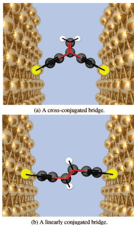
**Figure 1.** The bonding geometry of a molecule bridging source and drain electrodes controls whether the bridge is cross-conjugated (a) or linearly conjugated (b).
