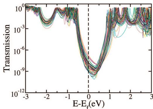
**Figure 7.** Transmission through **4** for 50 different geometries obtained from molecular dynamics calculations. Importantly, the antiresonance is present in all cases.
